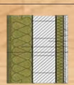
In order of comparison, the X-lam panel, the concrete panel and the punctured brick panel
